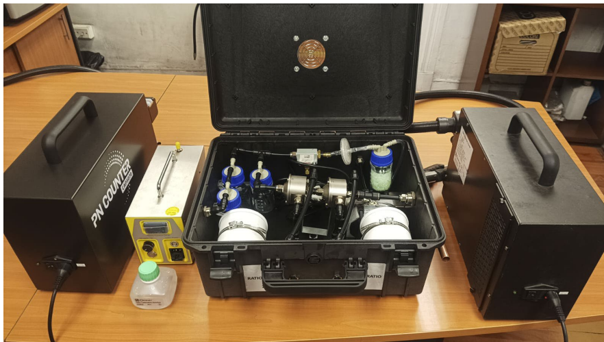
Calibration case with salt aerosol generator and reference counter
