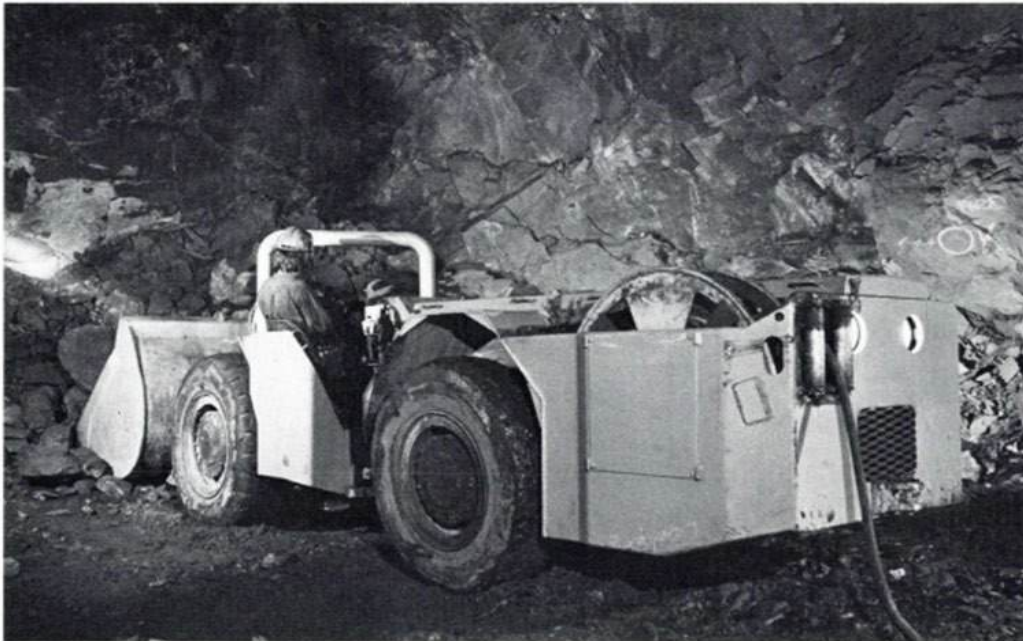
That's the new 2-yard electric scooptram , now in operation at Creighton mine. A new concept in load-haul-dump operation, the unit is operating in a cut-and-fill stoping complex on the 6600 level.
