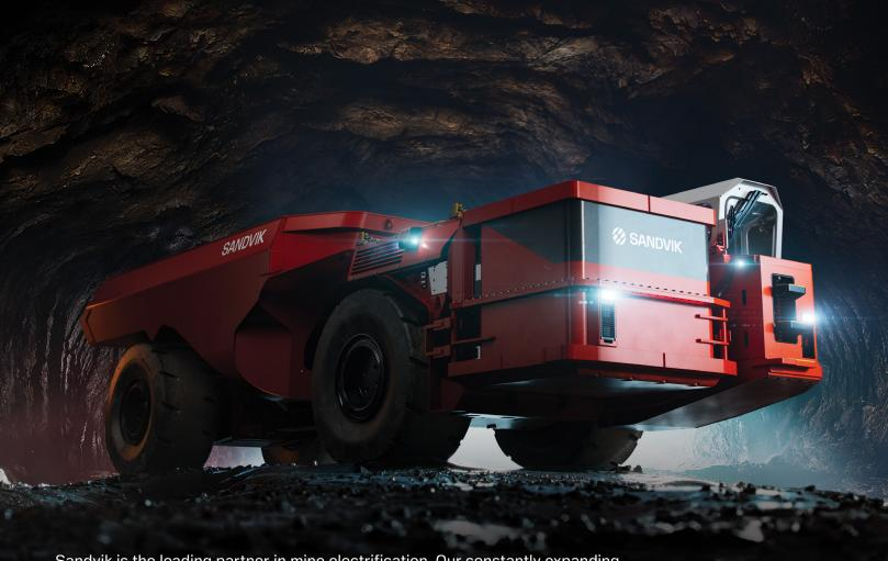
Sandvik is the leading partner in mine electrification. Our constantly expanding range of electric equipment produces zero diesel emissions and reduces ventilation and cooling needs in your mine. Our BEV loaders and trucks are designed from the ground up entirely around their battery system and electric driveline. The patented self-swapping battery system enables the industry's fastest and easiest pit stop.
