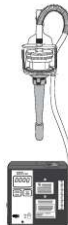
Figure 2. DPM Sampling Train with GS-1 Cyclone, Cassette Holder, and Universal PCXR4 Pump
