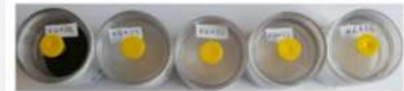
Figure 3.10: NIOSH 5610 filter cassette post-sampling, N428 - pre-filter sample, N429, 430, 432 and 433 - post-filter samples, 95C, 100C
