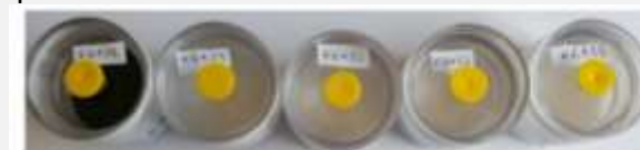
Figure 3.10: NIOSH 5040 filter canisters post sampling. 30428 - pre-filter sample, 30429, 403, 404 and 405 - post filter samples, 95% tests
