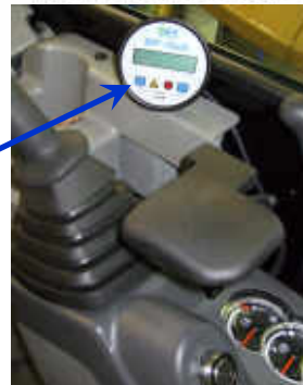
Alarm Indicator at the Drivers Seat or remotely controlled
