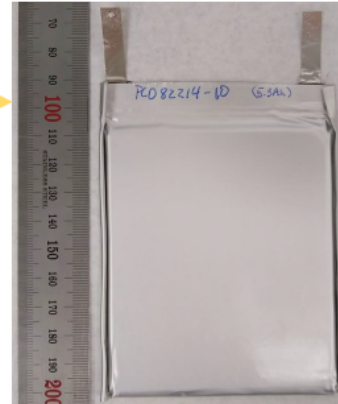
Photograph of 5.3Ah CAM-7/Graphite Cell*
