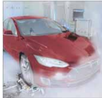
Cold Temperature Testing (-20 °C)
