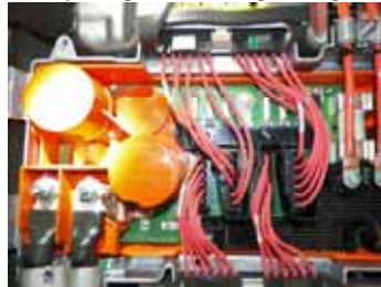
Voltage and Current Sensors on Junction Boxes and Contactors
