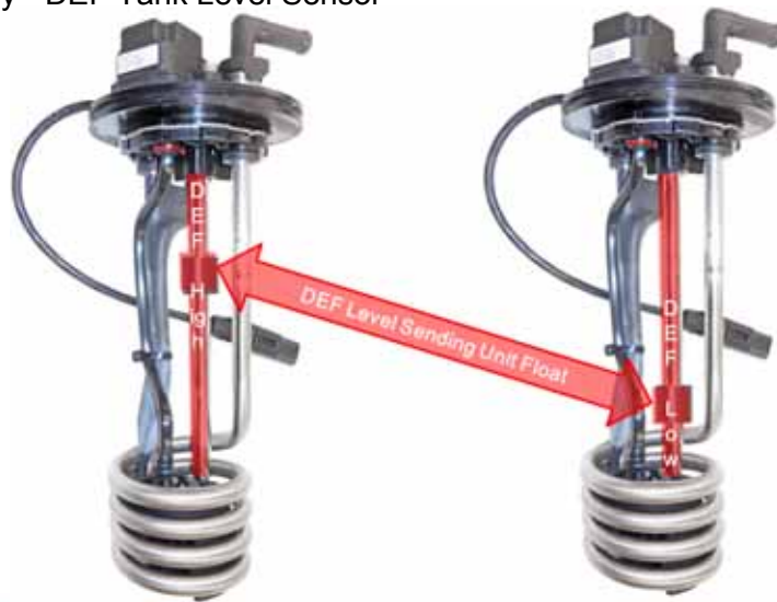
DEF Tank Assembly - DEF Tank Level Sensor
