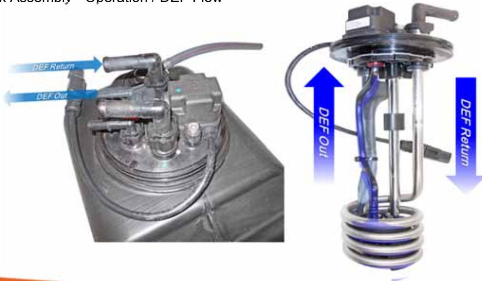
DEF Tank Assembly - Operation / DEF Flow
