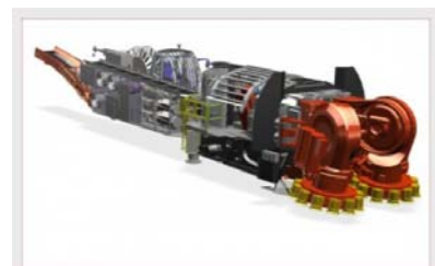
Sandvik's MX650 will be a mechanical excavation machine applying roller-disc undercutting technology
