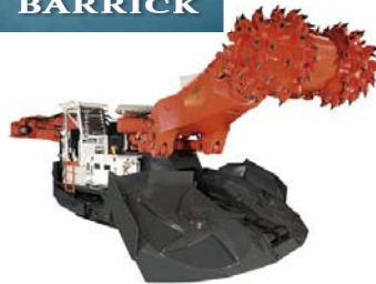
Sandvik's MX650 will be a mechanical excavation machine applying roller-disc undercutting technology
