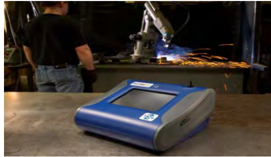
Desktop DustTrak DRX Aerosol Monitor Measuring welding shop exposures
