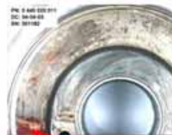
Fuel pump hsg deposits and corrosion from low use test
