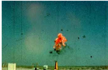
Detonation of treated JP-5 aviation fuel. Notice the much smaller smoke cloud.
