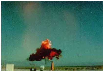
Detonation of Untreated JP-5 Aviation Fuel. Notice the size of the smoke cloud.
