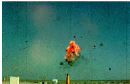
Detonation of treated JP-5 aviation fuel. Notice the much smaller smoke cloud.
