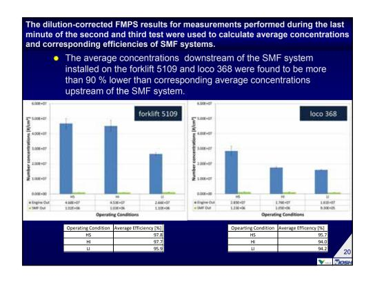
The FMPS size distribution measurements showed that the SMF systems installed on both vehicles not only dramatically reduced concentrations, but also changed size distributions of aerosols.
