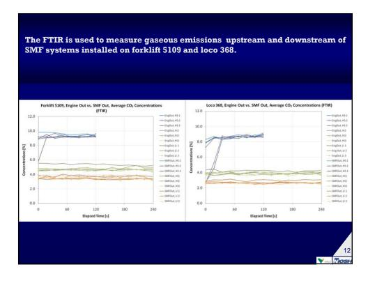
The results of FTIR measurements performed during the last minute of each test were used to calculate average CO,  $\rm CO_2$ , NO,  $\rm NO_2$ , and  $\rm NO_X$  concentrations.
