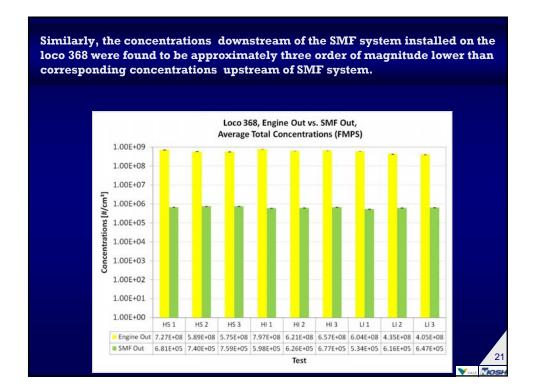
When compared with corresponding number concentrations measured upstream of those systems, the number concentrations measured after SMF systems were found to be at least 80 times lower.
