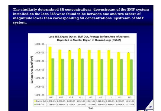
When compared with corresponding surface area concentrations measured upstream of those systems, the surface area concentrations measured after SMF systems were found to be at least 57% lower.
