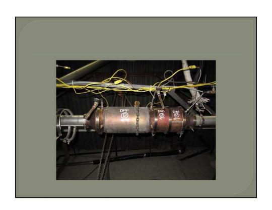
**System A** – 3 components consisting of cordierite DOC, cordierite DPF and a cordierite NO2 suppression catalyst
