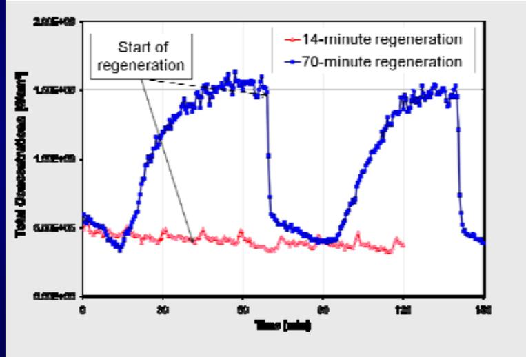
For R100 conditions during the 70-min. regeneration cycle, size distribution measurements showed a gradual increase in number of nucleation mode particles and decrease in number of accumulation mode particles after the electrical regeneration of SM DPF.
