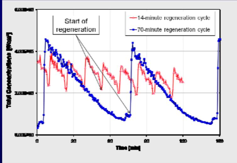
The accumulation of aerosols in the media results in lower peak concentrations of aerosols at the end than at the beginning of the regeneration cycle.
