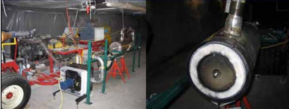
Air-to-air heat exchanger
