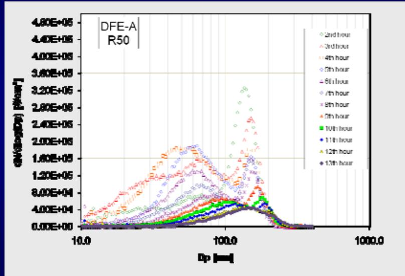
Similarly, total number concentrations of aerosols in mine air during test of the Cordierite DPF system decreased gradually with accumulation of DPM in filter media.
