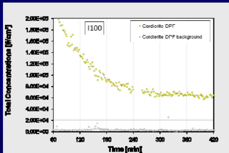
Total mass concentrations of aerosols in mine air during a similar test (only 120 min) of Cordierite DPF decreased with accumulation of DPM in DPF.
