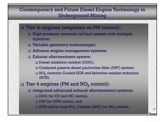
Future of diesel engine and exhaust aftertreatment technology looks bright, but optimization is needed for underground mining application.
