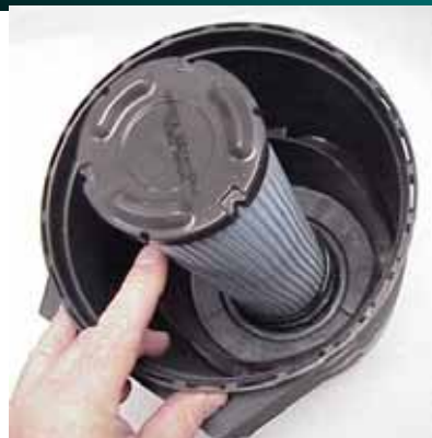
Fig. V-4. Structure of double element air cleaner
