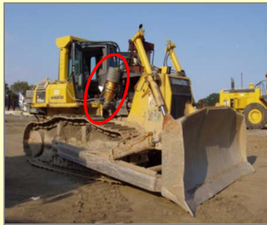
Laminar Flow Element (LFE) for intake air flow measurement
