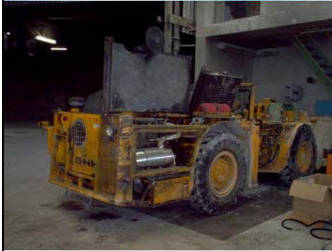
GHH LF 41 wheel loader with diesel burner DPF
