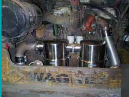
Wagner ST-8 Loader DDC Series 60 with Combifilter Model 2xS18
