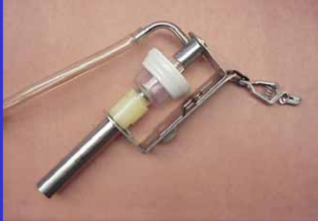
DPM Filter Cassette Mounted On Cyclone In Lapel Holder
