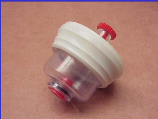
SKC DPM filter cassette with submicron impactor and tandem quartz fiber filters
