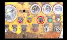
It may not be directly attributed to a plugged filter system should these indicator lights signal. It may be attributed to other engine functions.
