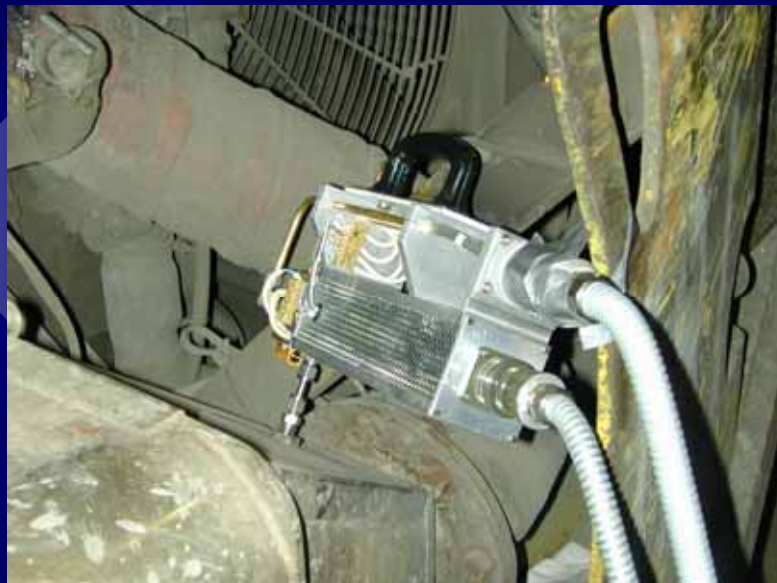
Figure 12. Dilution System Probe Installed Upstream of the Knitted Fiber Filter Fitted on Truck #3
