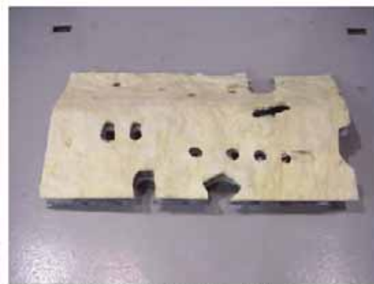
Figure 2: Rear side of enclosure with fiberglass
