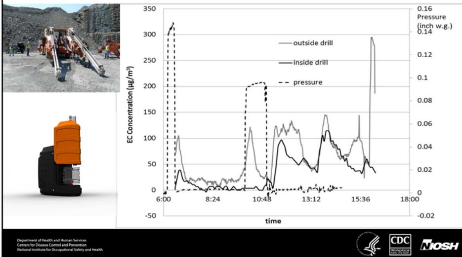
The long term measurements showed that the efficiency in reducing exposures of the miners to EC was substantially higher during the periods when doors and windows were completely closed. 18
