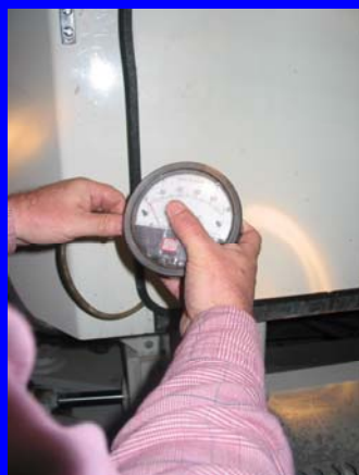
Magnehelic gage with rubber hose extending into cab
