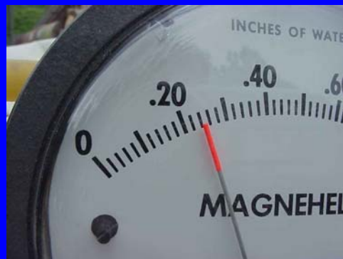
Magnehelic gage should register + 0.20" WG or more
